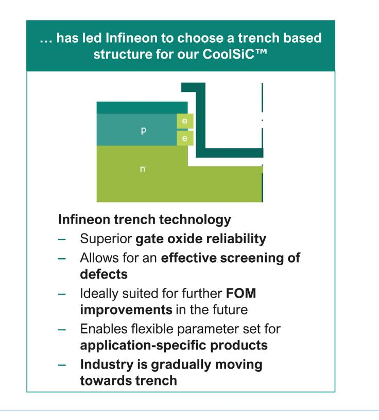
Additionally, the technology addresses a common challenge in power electronics: parasitic turn-on. CoolSiC<sup>™</sup> devices are resistant to these unwanted switching events because of their higher gate-source threshold voltage as well as the improved ratio of CGD and CDS capacitances. This allows engineers to operate the device at a gate-source voltage turn-off of O volts, removing the need for negative gate voltages and making system design and integration easier.
