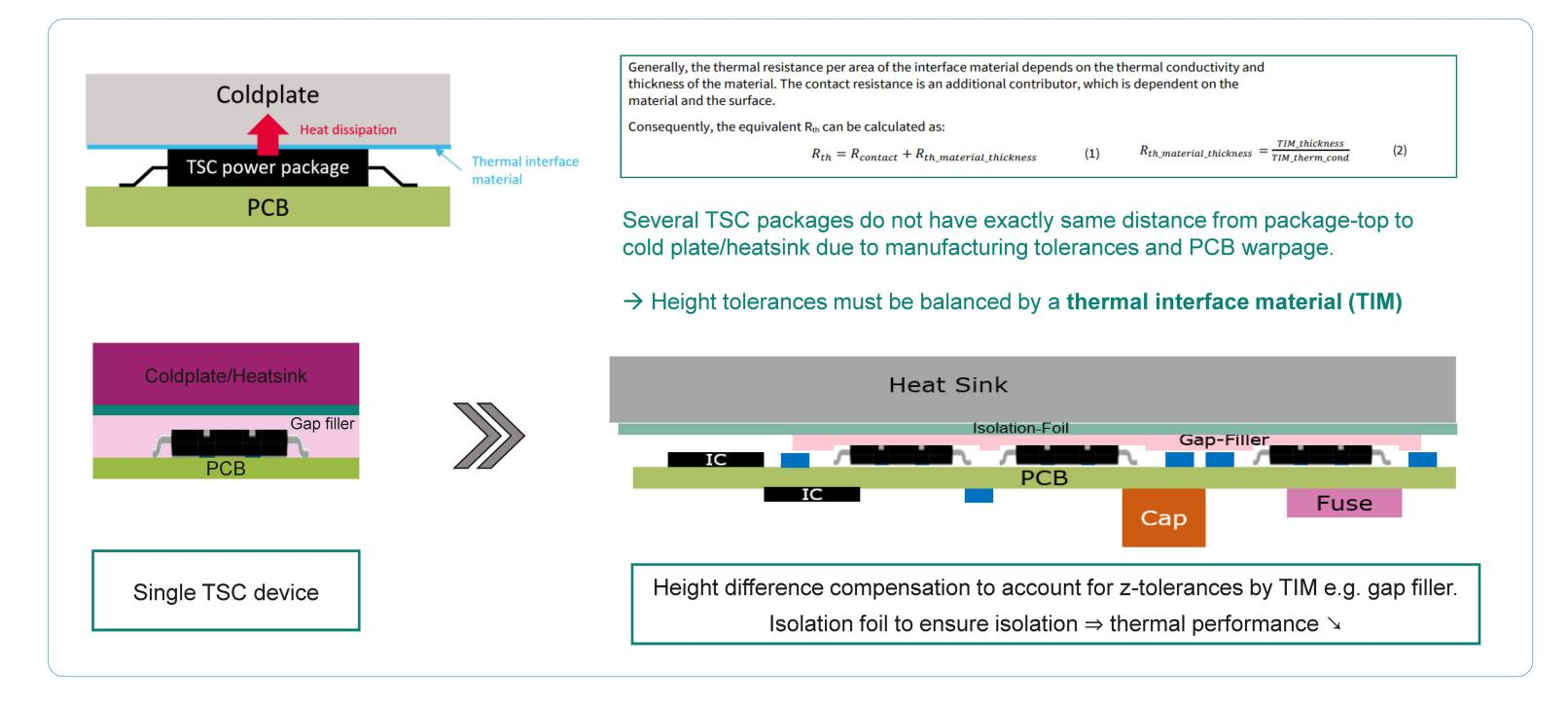
System designers must consider multiple factors: package height variations, potential PCB warpage under mounting pressure, electrical isolation requirements, and mechanical assembly constraints. Each application requires careful evaluation to optimize the thermal solution.
